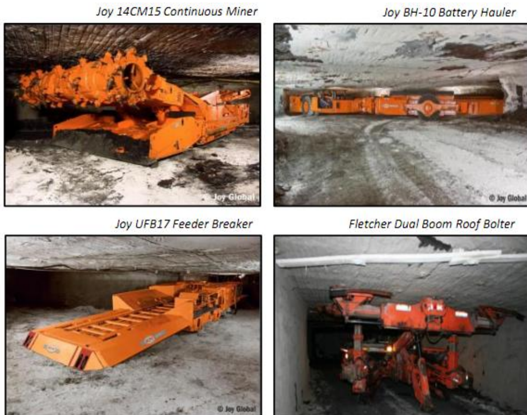
Figure 15: Typical Underground Super-Section Mining Equipment
