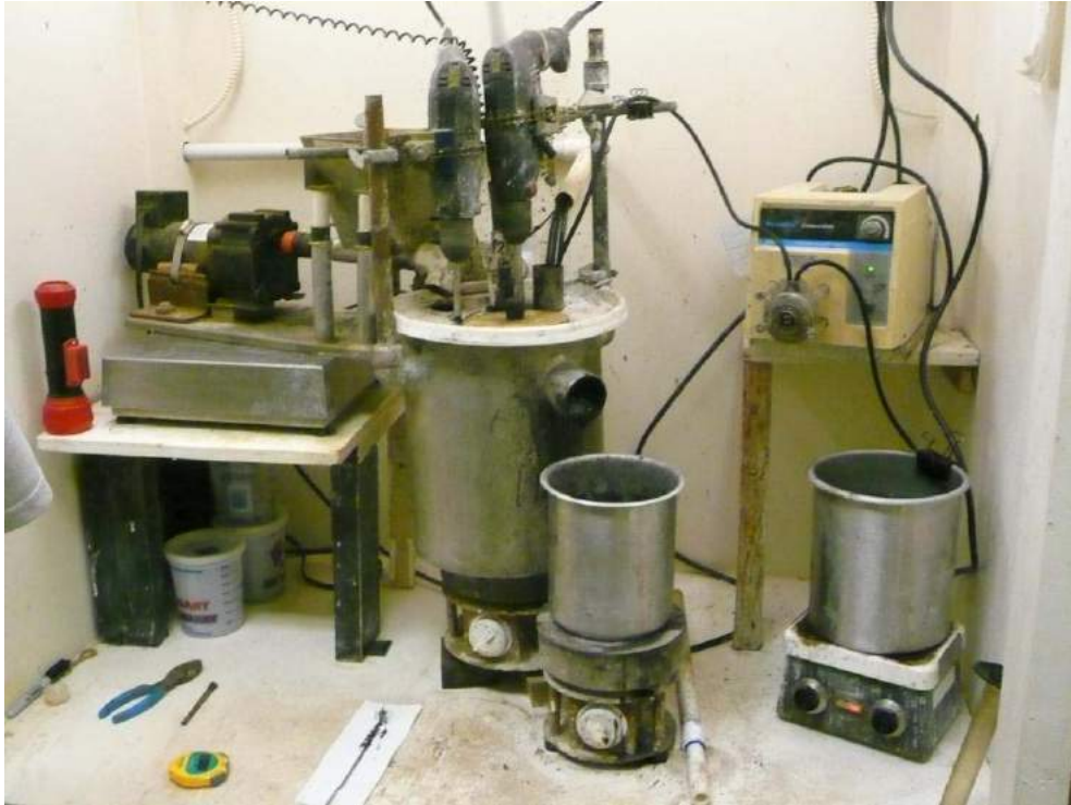
Figure 13-2. Acidulation Pilot Plant for Processing Lower Phosphate Zone Mineralization
