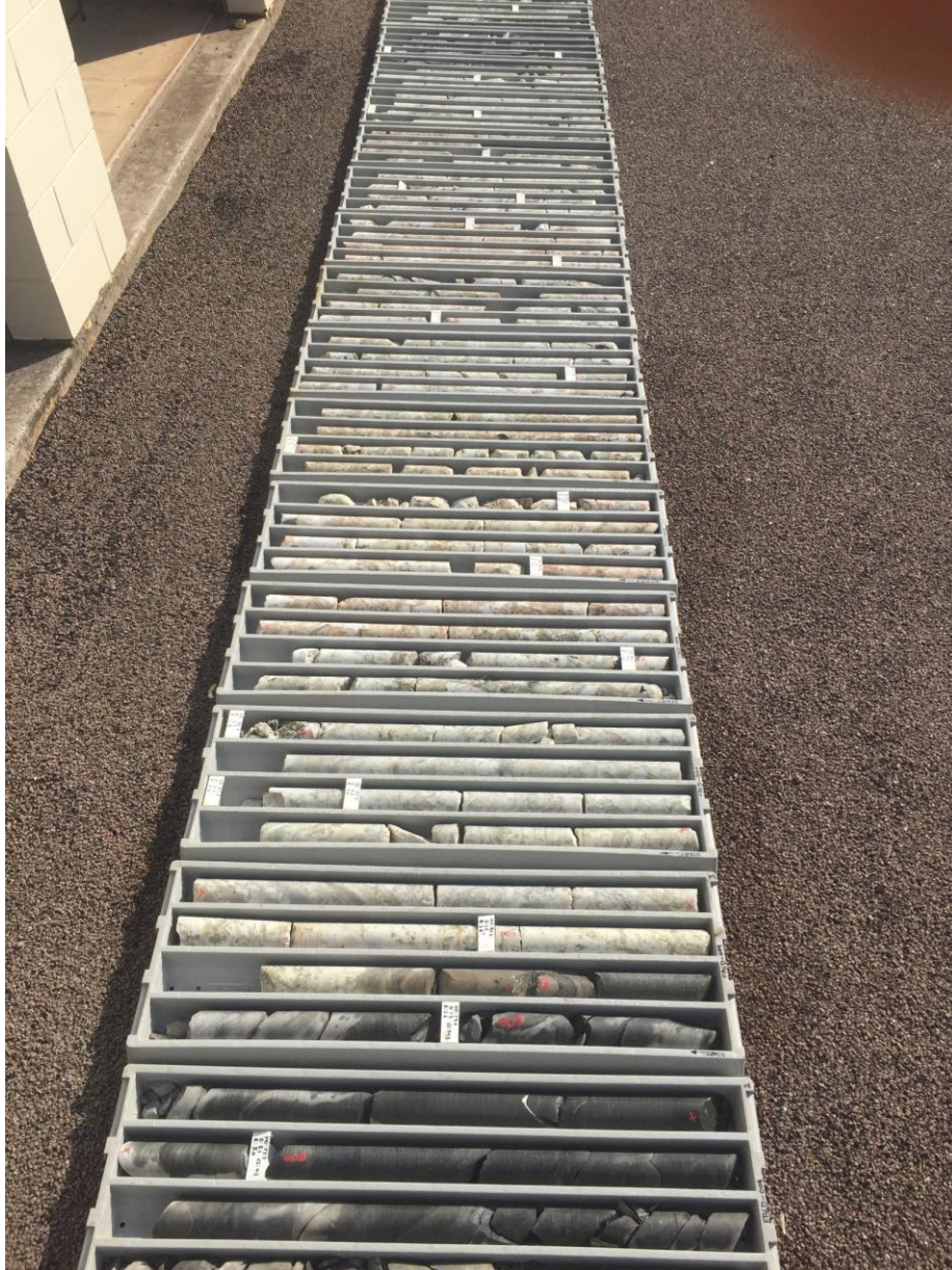
Figure 4. BP33 Spodumene Pegmatite in drillcore (79m-120m FRCD004) BP33, Finniss Lithium Project.
