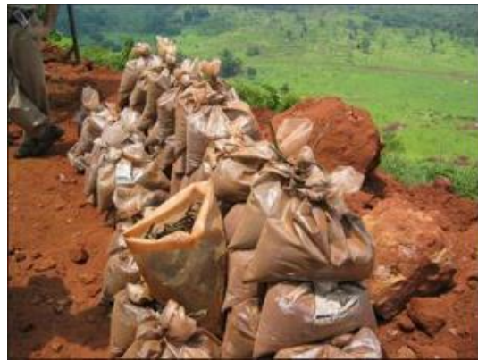
Bagged and labelled RC samples at drill pad, ready for transport to farm
