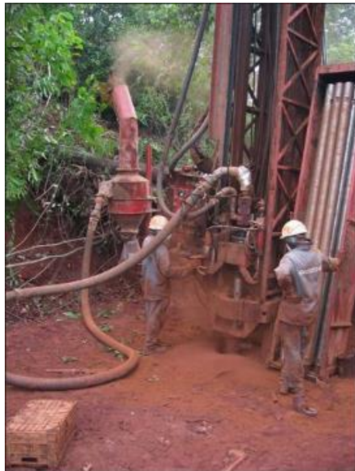
Infill RC operations – Prospector W750 articulated rig at V1 LT725W
