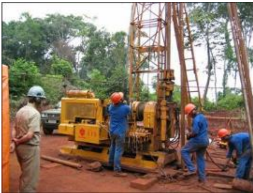
Large diameter coring operations – pulling the core barrel at FM 78
